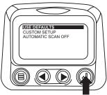
7. A message indicating the "Single Engine" parameter display parameters are reset to the factory defaults will be displayed, then the display will return to the "Custom Setup" menu.
